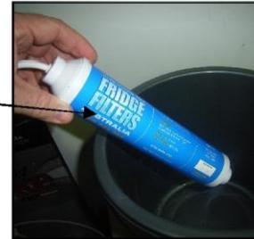
3. Take the new filter, making sure the flow direction is correct and insert the inlet side only, the line will go in approx 5 – 10mm and you will feel it hit home.
