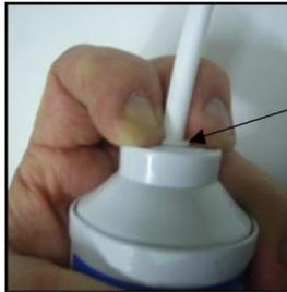
You can use your fingers or a firm edged object to hold down the locking collar, this will allow the hose to easily slide out.
