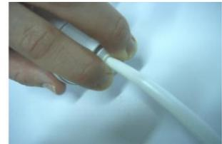
Unscrew your fitting and remove hose from old filter. Follow steps 3 – 5 for replacing filters as noted above **IMPORTANT:** the end of the hose needs to be neatly cut and maintain its circular structure. If the hose is damaged in any way use a sharp Stanley knife to cut off the unsuitable portion of hose.
